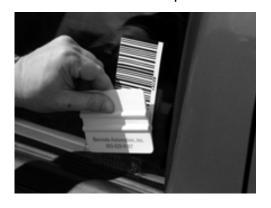
4. Place squeegee at top of decal. Press firmly against window and run it smoothly down the decal where the backing was peeled back
